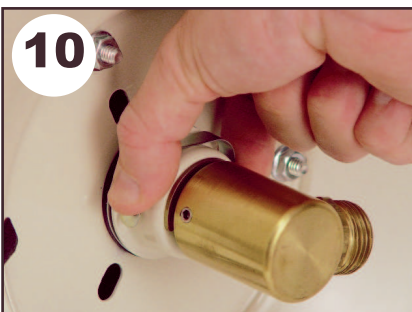
10 Secure new assembly to the reel by firmly pushing the "tabs" of the snap button into the holes.
